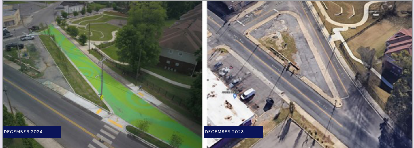
EARLY STAGE INVESTMENTS (ESI) ON KERR AVE AND GAITHER ST INCLUDED THE INSTALLATION OF CURBED AND LANDSCAPED MEDIANS AND MIDBLOCK CROSSING AND ADA ACCESSIBLE CURB RAMPS, REMOVABLE BOLLARDS AND PLANTERS FOR PEDESTRIAN SAFETY.
